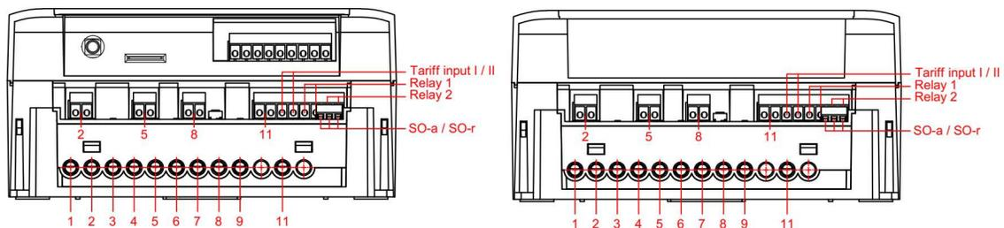
**Figure 2.4** Meter terminal connector's labels (with GPRS modem left, without modem right)
