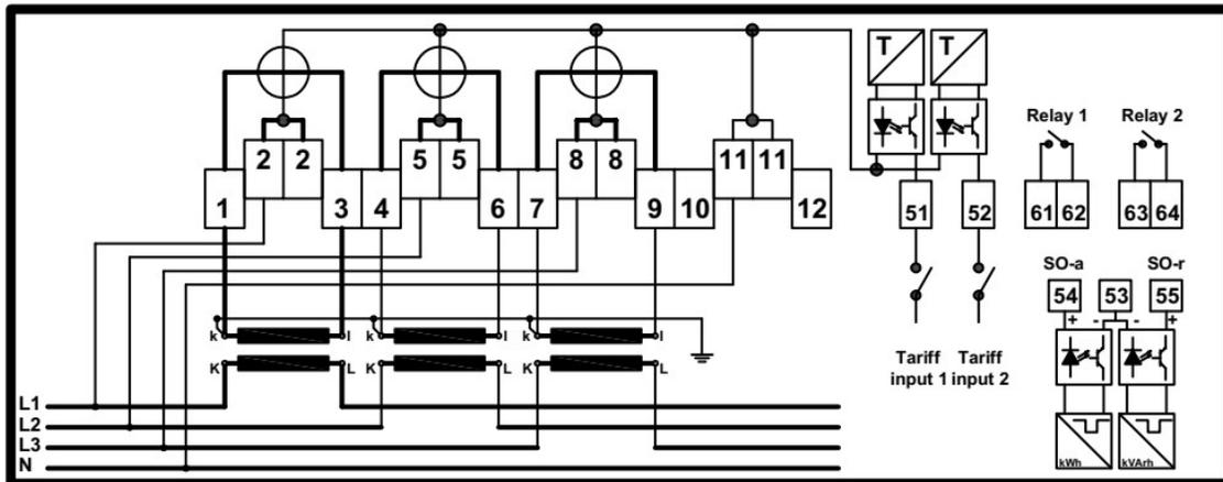
Figure 2.7 Current transformer operated meter connection scheme
